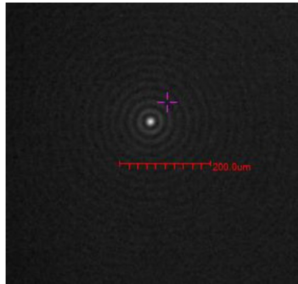
FIGURE 1a. Reflected spot produced by a CGH pattern of equally spaced concentric rings, or a pattern simulating an axicon.
