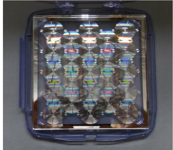
FIGURE 6. A 6" photomask CGH with a close packed hexagonal array of Fresnel zone patterns on 28 mm centers 5 . The interferogram in Fig. 2a is of one of these patterns.
