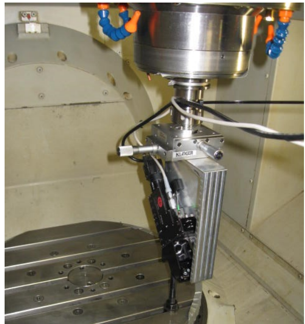
FIGURE 2. BCF centered on ball mounted to work table (above). BCF and PSM mounted on the spindle of a Mori Seiki NMV5000 showing orientation of BCF to machine X axis (lower).
